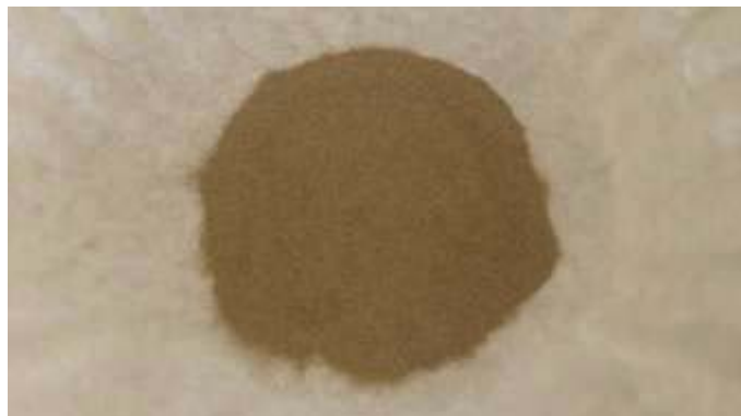
Fine grit removed by PISTA® system.
