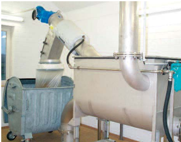
Tank-mounted ROTAMAT® Rotary Drum Fine Screen Ro 2 ...
